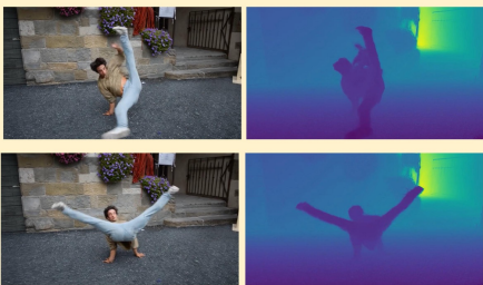
Render RGBs and Depths with GS-Splatting and supervise with observed images and inferred foundation mono-depths
